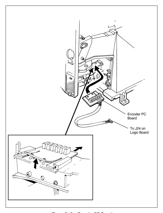
Figure 5-12a Encoder PC Board
